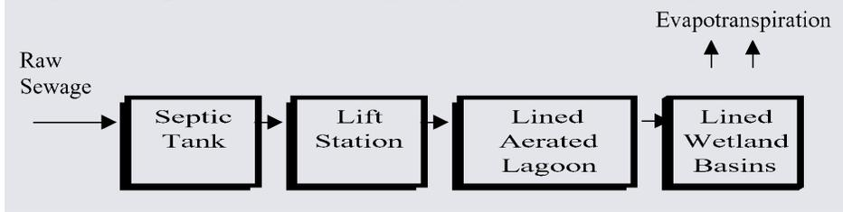
There are no limitations on the geometry of the basins since they are a non-discharge system. The basins can be curved to provide a natural look depending on the site conditions. Wetlands generally are designed with shallow level basins.
