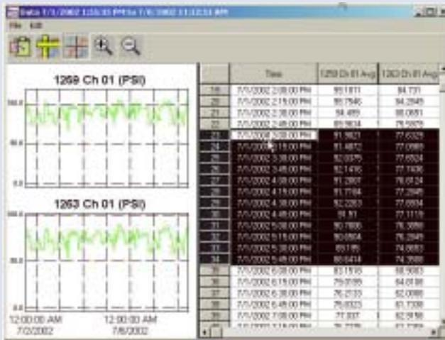
In time series analysis you can study your system over an extended period of time. Fill and drain cycles of tanks, pump and valve response, as well as daily fluctuations in usage, can all be simulated using time-series analysis. The HPR easily collects and exports these data to your modeling software package.
