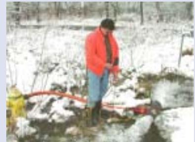
Use your Telog Palm DTU to observe the static pressure at the upstream and downstream hydrants
