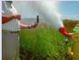
Attach an HPR unit to the residual hydrant and an HPR unit with diffuser to the flow hydrant. Using your Telog Palm DTU, you will be able to do on-the-spot pressure analysis. All data is stored in the Palm for further viewing and analysis on your PC running Telogers for Windows software.
