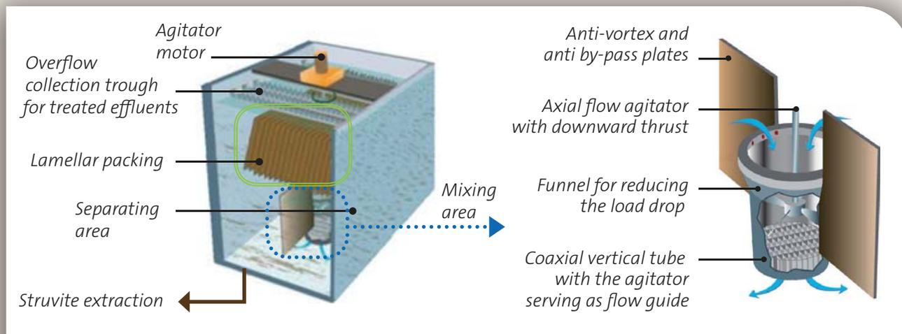
Turbomix™ is patented by Veolia Water Technologies. It encourages crystallization and growth of struvite pellets and it allows for optimum use of reactive products with a short reaction time, thereby reducing system footprint.
