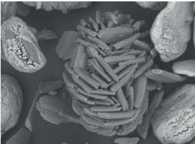
*Struvite pellets produced in a Struvia™ reactor*
