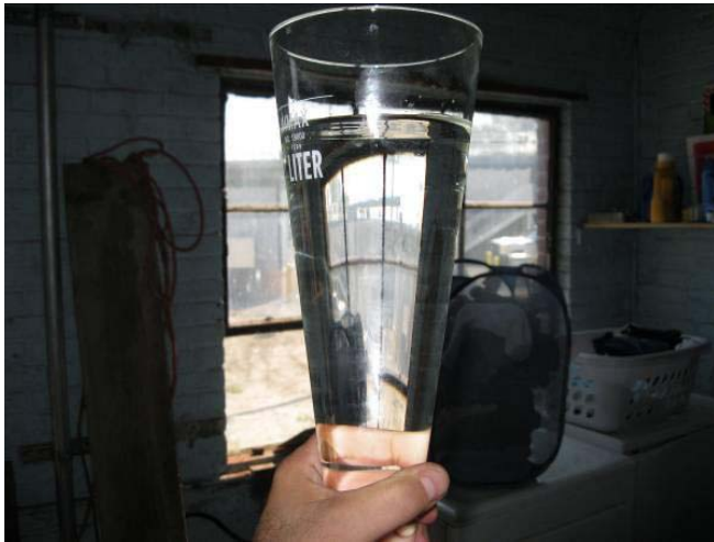
Figure 3: Permeate produced from a membrane thickening aerobic digestion process
