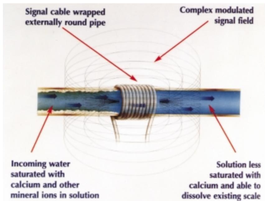
◀ Magnetic and electronic descaling systems alter the shape of the crystals to reduce the adherence and build-up of deposits on the pipewall.
