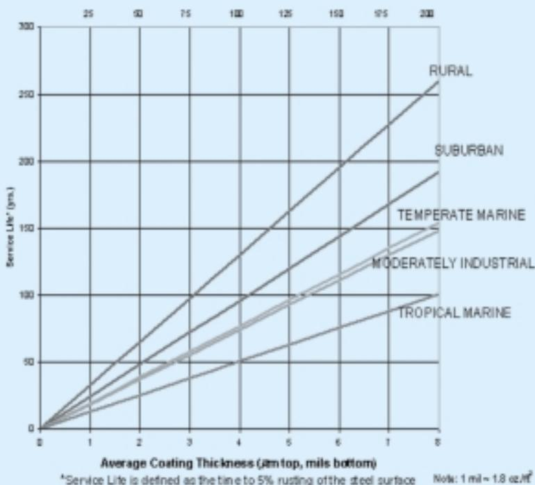
in-line process applies about 0.9 mils (0.5 oz/ft<sup>2</sup>). As the Service Life chart (Figure 1) indicates, the batch-process-produced zinc coating will perform in use without maintenance approximately three times longer than the in-line-produced zinc coating.
