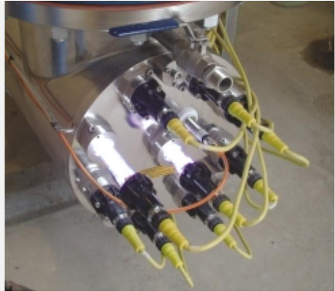
Ultraviolet light inactivates microbes by damaging their DNA, thereby preventing the microbes' ability to replicate. Unlike chemical disinfectants, UV disinfection leaves no harmful byproducts and does not impart any taste or odor to the water supply.
