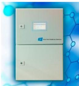
An alternative TOC analytical method is the UV correlation technique performed by the ECD UV-6 Analyzer.
