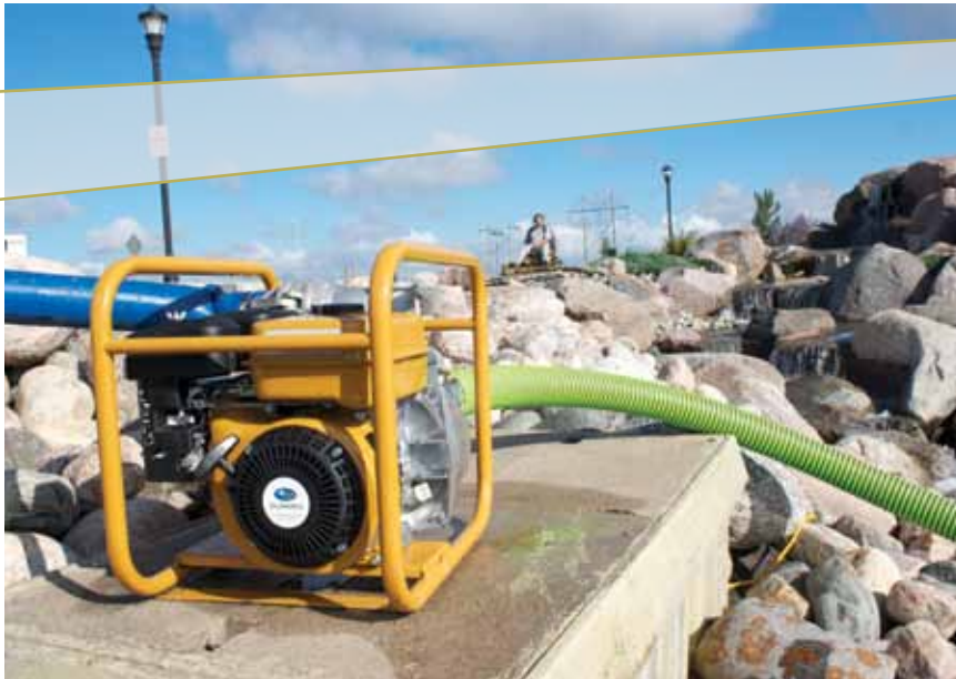
A semi-trash pump moves muddy water from a jobsite. Semi-trash and trash pumps' impellers are made with thicker veins than those in standard centrifugal pumps, which enables them to move larger debris.
