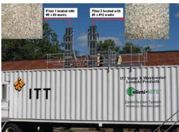
Pilot trailer, and media loaded in the filter columns.
