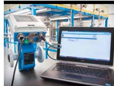
For field verification, a technician connects a laptop PC to the flowmeter via an Ethernet connection, and accesses the meter via an integrated Web server. The flowmeter does not have to be removed for this procedure. The same procedure can also be done from a remote PC.
