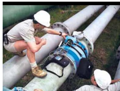
To perform external verification, a technician connects a verification tool and a simulation box to an installed flowmeter.
