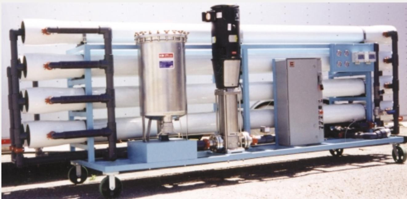
Nanofiltration has some benefits that micro and ultrafiltration do not. These benefits include removal of uranium, lead, pesticides and herbicides from the water stream.
