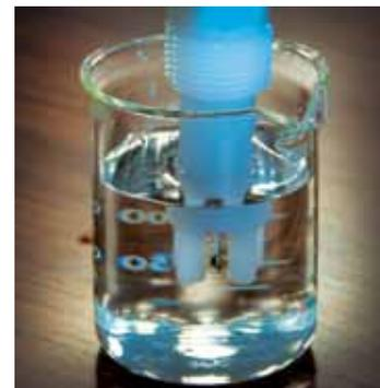
Figure 2: A pH sensor being kept wet in tap water
