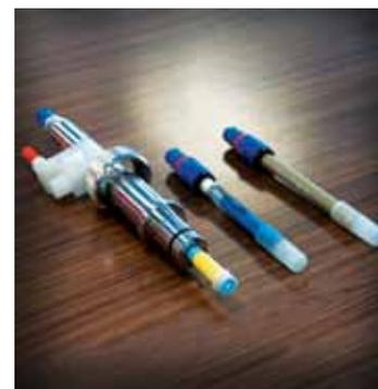
Figure 3: Store pH sensors with manufacturer's supplied boot/shipping cap or in beakers with storage solution.
