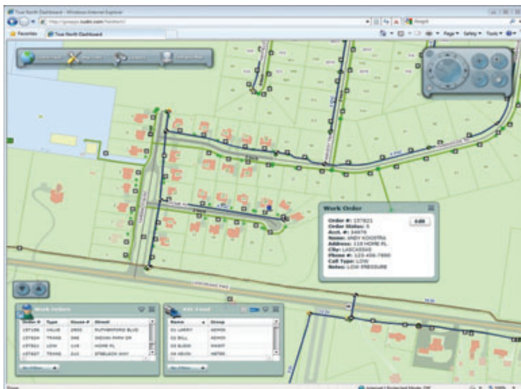
GIS can overlay and combine different kinds of information on a single map that summarizes and identifies customer locations, work orders and water utility assets.
